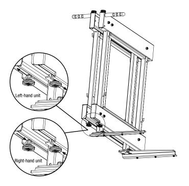
Attach center assembly (A) with feet to the slide base (E) with remaining 6 - M5 x 8mm (G) screws.
