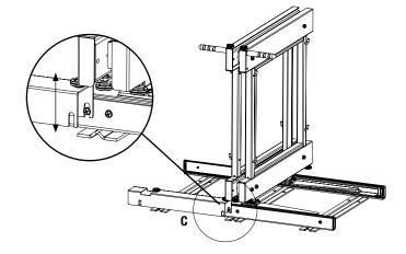
Position and align completed unit in cabinet. Recommended to place completed unit at least 2.5" from side of cabinet and 2.75" from front edge of cabinet. Temporarily place at least one basket (F) on each side of the frame assembly and verify that both baskets will clear the opening when operating the product.
