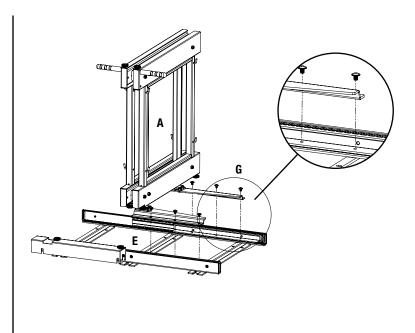
Attach front guide stop channel (C), replacing 2 - short M4 screws with 2 - longer M4 x 8mm (H) screws.
