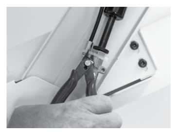
**4** Cut the zip ties holding the cable to the top and bottom of the old cylinder.
