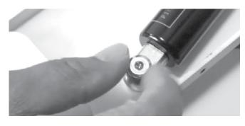
**7** Reinstall the cylinder attachment bolts, both top and bottom, to *finger tightness only*.
