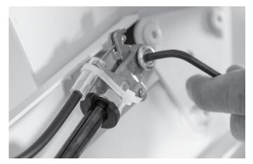
**9** Using the 4mm hex wrench, tighten the upper and lower cylinder bolts to *finger pressure only*.
