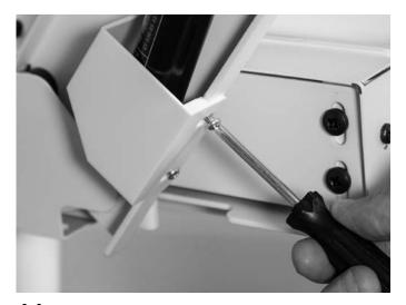
**11** Reinstall both new rear cylinder shrouds.
