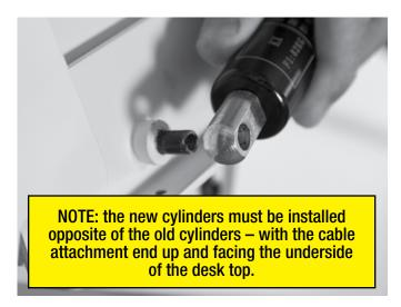
**6** Replace with one of the new cylinders. Start by attaching the cable end eyelet to the upper frame post and then by squeezing the height adjustment lever, adjust the desk height to match the new cylinder length, placing the lower cylinder eyelet over the bottom post.
