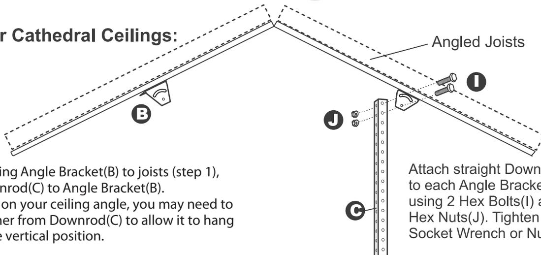
After installing Angle Bracket(B) to joists (step 1), attach Downrod(C) to Angle Bracket(B). Depending on your ceiling angle, you may need to cut the corner from Downrod(C) to allow it to hang down in the vertical position.
