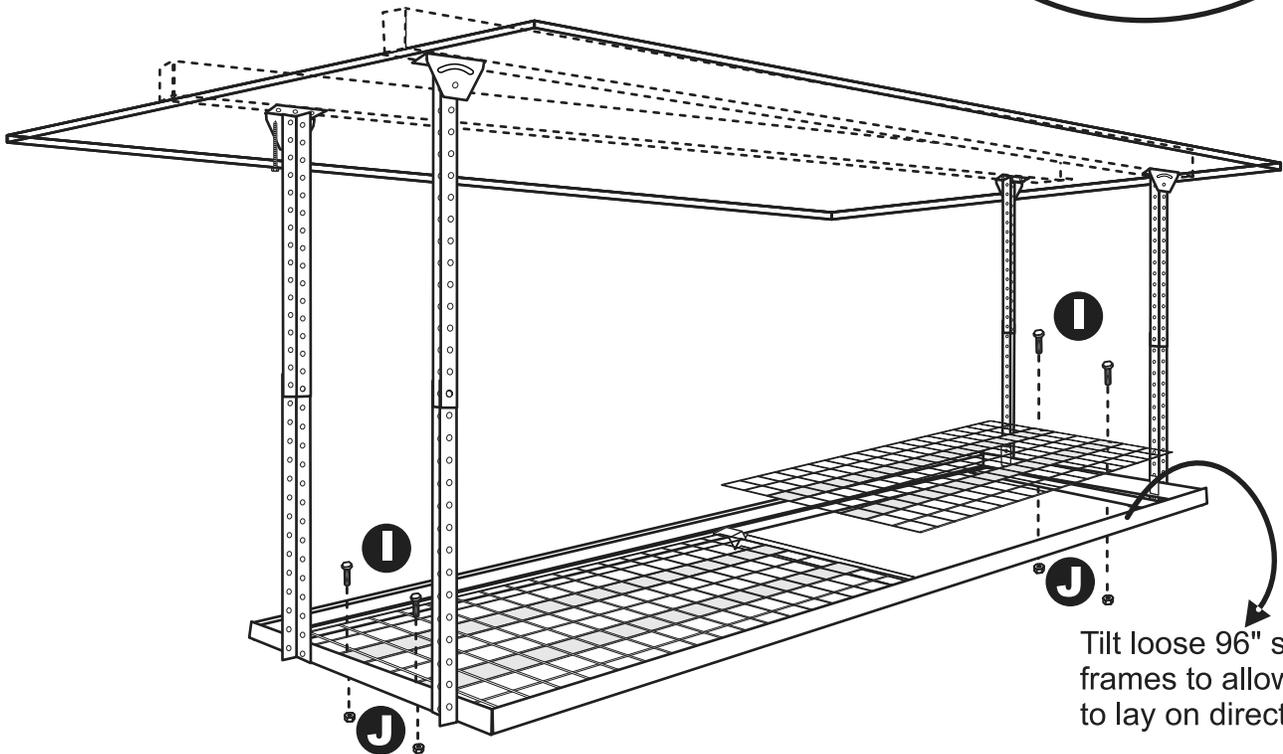
Tilt loose 96" support frames to allow grids to lay on directly on ledge.
