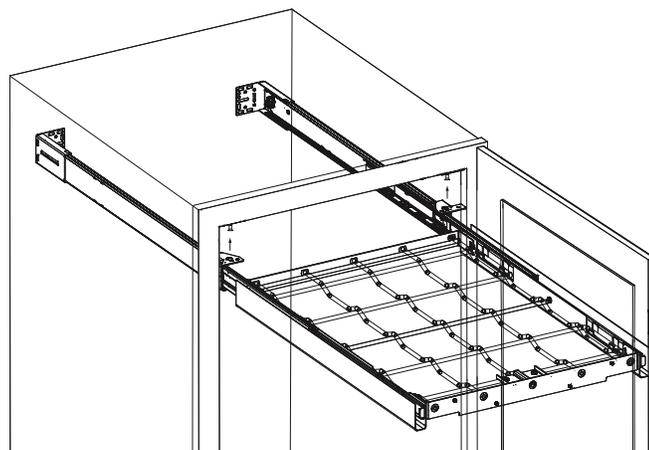
**4B.** Lift rear of pan rack assembly up until shaded hole on rear mounting bracket (4B) lines up with both pilot holes. Screw 1 – #8 x ½" sheet metal screw into each pilot hole so they are secure. Choose any round hole on each rear mounting bracket and screw 1 – #8 x ½" sheet metal screw into each bracket so they are secure.
